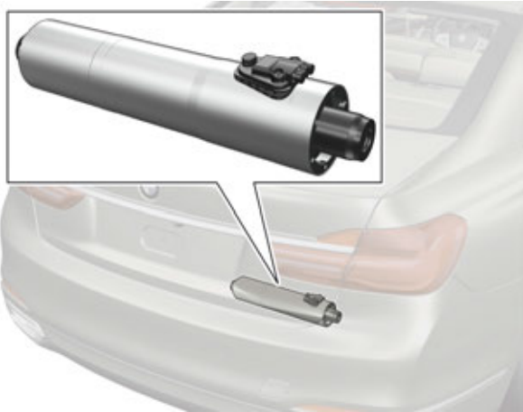
Electric Active Roll Stabilization rear, EARSH
